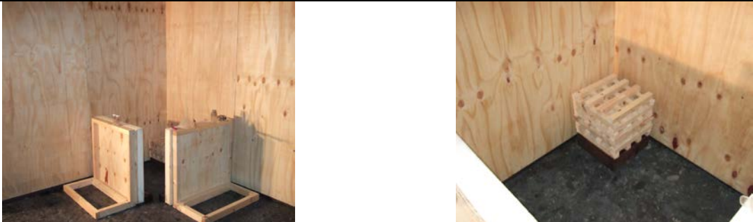
Photographs of ignition and fuel package before a test
