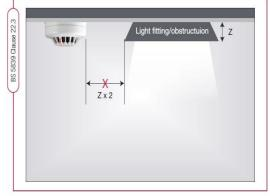
For obstructions less than 250mm deep never mount devices closer than twice the depth of light fittings or other obstructions in the ceiling.
